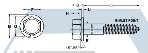
Length of a hex flange lag screw (L) is measured from the underhead bearing surface to the extreme end of the screw. Minimum thread length is 1/2 length of the screw plus 0.50 inch or 6 inches, whichever is shorter.
