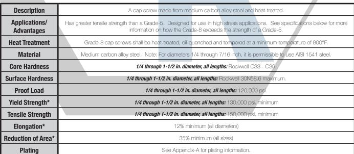
\*These properties are tested only on machined specimens when the testing machine cannot provide for full testing of the parts.
